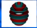
Figure 1. This image shows the structure of the spherical cusp with each concentric layer representing a low resistance coil with the blue coils representing positive current flow and the red coils representing negative current flow.
