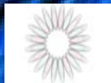
Figure 3. This image provides a rough sketch of the magnetic field for the spherical cusp with the magnetic field lines illustrating the magnetic contour as a result of positive and negative current flow in the blue and red coils.
