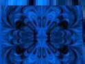
Figure 5. This image shows the contour of the magnetic field for a spherical cusp with ten concentric loops of current with each segment representing current in a direction opposite to the direction of each of the adjacent segments.
